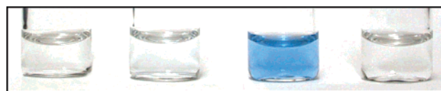
Figure 2. Selective color change in response to Hcy in solutions of MV^{2+} . Left to right: no added analyte, cysteine, homocysteine, and glutathione.
